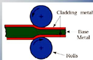
Fig. The roll bonding or cladding process
