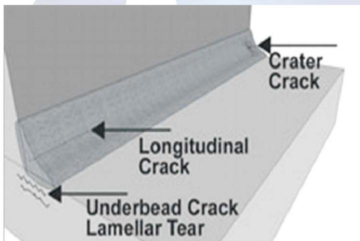
The most common cause for cracking has been attributed to lack of pre heating in thick sections particularly in cold weather.
