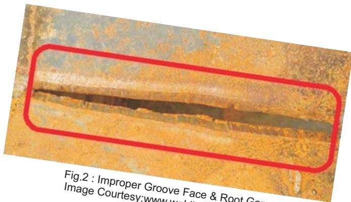
Fig.2 : Improper Groove Face & Root Gap
